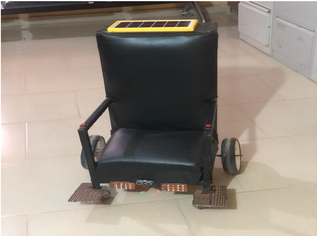
Figure 15: The designed and constructed low-cost smart solar-powered wheelchair.
