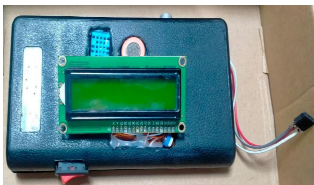
Figure 9: The photograph of the designed, constructed and cased IoT-based neonatal incubator assistant for real-time monitoring of preterm infant neonatal incubator.
