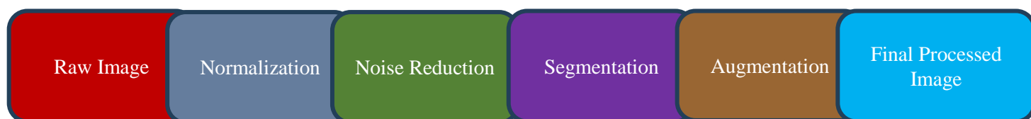
Figure 5: Preprocessing Workflow for Microscopic Images
