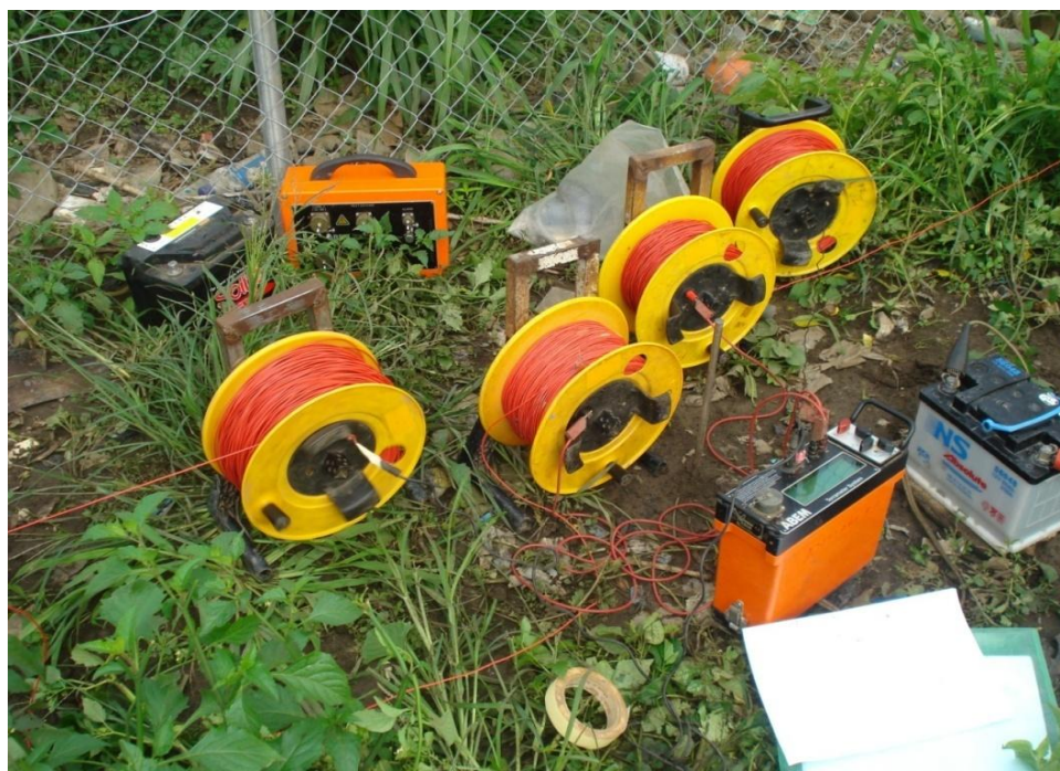
Figure 1: ABEM SAS 1000 Terrameter and its accessories.
