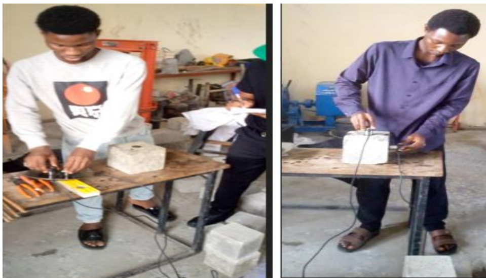
Figure 3: Schematic representation of UPV test configurations showing Direct, Semi-Direct, and Indirect measurement setups on a concrete cube.
