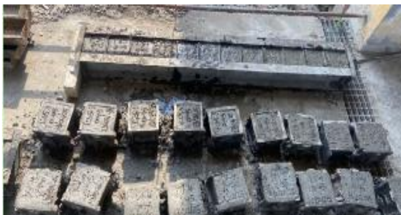
Figure 1: Casting of Concrete Specimens for Experimental Testing
