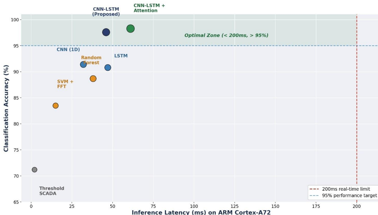
Figure 11. Accuracy vs. Inference Latency Trade-off (Edge deployment: ARM Cortex-A72, TFLite INT8 quantisation; green zone = optimal for real-time Nigerian pipeline deployment; all proposed models fall within the 200ms real-time constraint)
