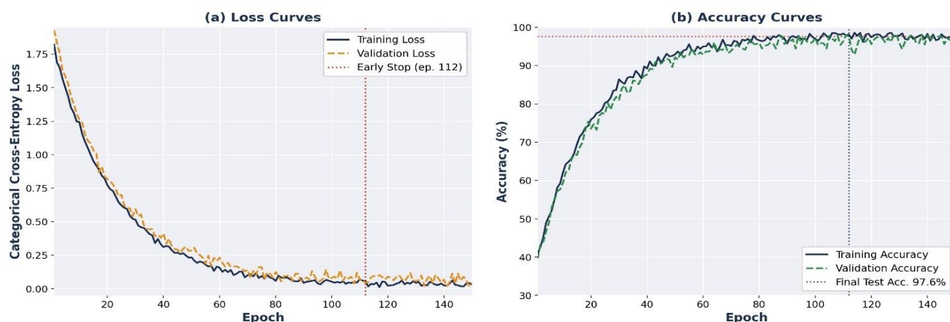
Figure 10. CNN-LSTM Training and Validation Curves (a) Categorical cross-entropy loss; (b) Classification accuracy. Adam optimiser, lr=1e-3 , ReduceLROnPlateau, early stopping at epoch 112 (patience=20, max 150 epochs).
