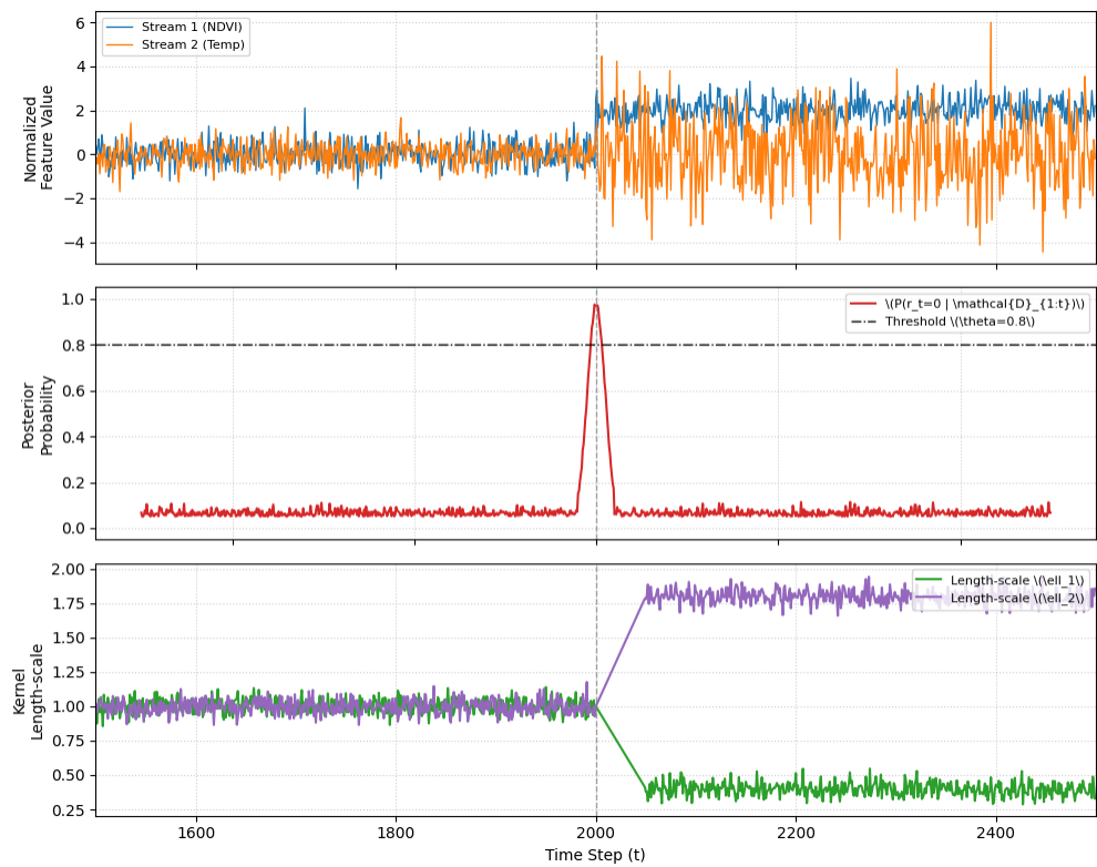
Figure 3. Temporal dynamics of input features, run-length variables, and adaptive kernel length-scales demonstrating immediate recalibration upon structural shifts.
